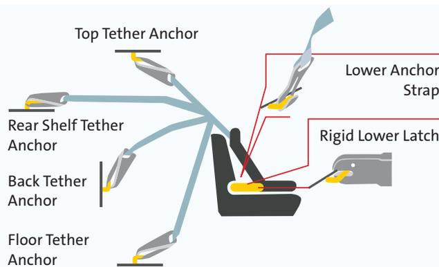
The lower anchor strap and rigid lower latch as shown are used **ONLY** in car seats fitted with ISOFIX connectors.
