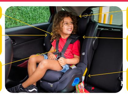
Ensure rear tether strap is secured to the correct anchor point.
